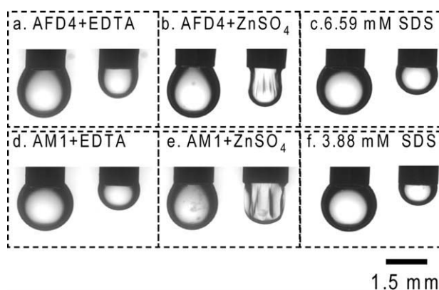
Figure 3. Response of a pendant water droplet in Miglyol 812 oil during interfacial contraction in the presence of different surfactant formulations.
